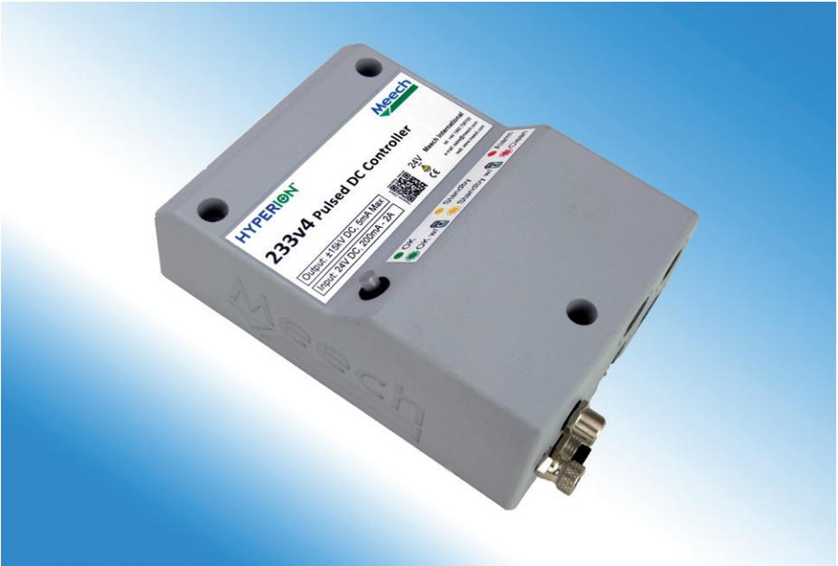
The Hyperion 233v4 Pulsed DC Controller is a compact and powerful 15kV controller. It was principally designed to directly power two Meech pulsed DC ionisers. If more ionisers are required, they can be connected via splitters.
