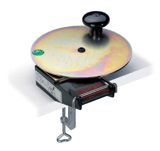
The AT-60 is a preparing device for skiving (grind to a thin wedge for a glued Thermofix joint) of Habasit belts and tapes up to a width of 60 mm / 2.4 in. and a thickness of 2 mm / 0.08 in.. The belt / tape is clamped and stuck on a steel plate. It is ground manually be means of a skiving disc. Adjustment is done with two different settings.
