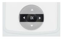
Please note the OK button in the centre of the toggle is redundant and has no function on the BarMaster.
