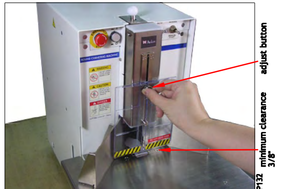
Loosen the adjust button of safety protector, move it down to the bottom and lock it. Keep the safety protector and work desk minimum clearance 3/8".
