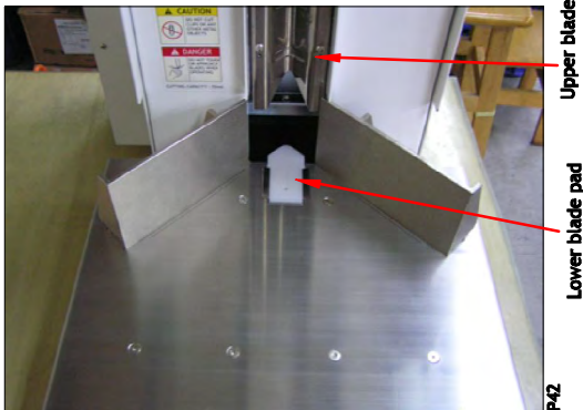
Above figure show the ready position for right and left side guide.
