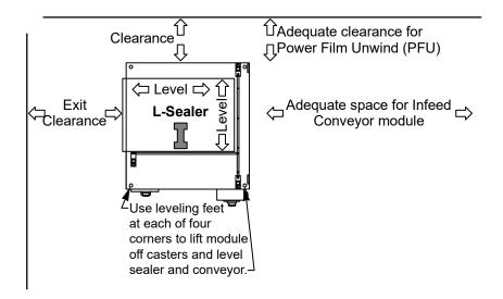
II. Next, bring the PFU/Infeed Conveyor/Inverter module up next to and in position with the L-Sealer/Exit Conveyor module. Note that there are attaching flanges welded to the base of the PFU/Infeed Conveyor/Inverter module, with bolt holes that must align with bolt holes in the base of the L-Sealer/Exit Conveyor module. When the unit is in position, use chock blocks to block the casters and secure it from moving.
