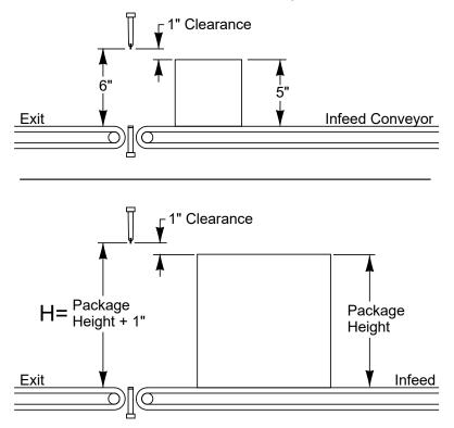
Similarly, allow approximately the same distance, H, between packages, so that the seals occur a distance  $D = \frac{1}{2} \times H$  before and after each package.
