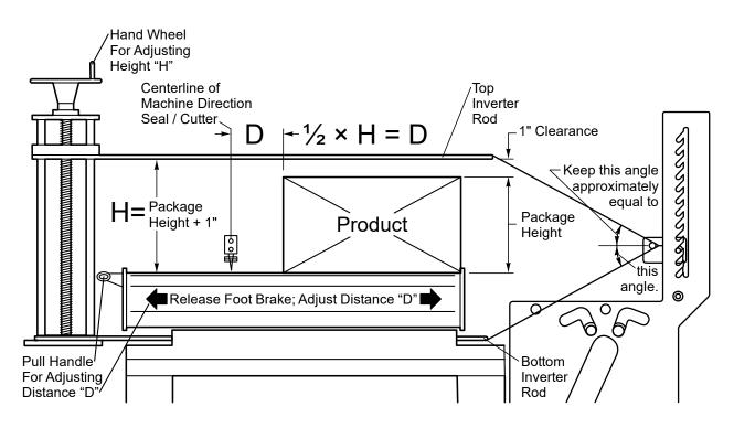
9. To adjust the infeed conveyor position for the width of the product package, release the locking foot near the center of the conveyor and the conveyor can be moved freely front to back. Re-engage the locking foot when the conveyor is positioned correctly.
