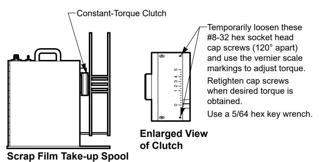
To adjust the clutch torque, temporarily loosen the #8-32 hex socket head cap screws. (Screws are located 120° apart.) Use the Vernier scale markings to adjust the torque. When the desired torque is obtained, retighten the socket head cap screws. Use a 5/64" hex key wrench.
