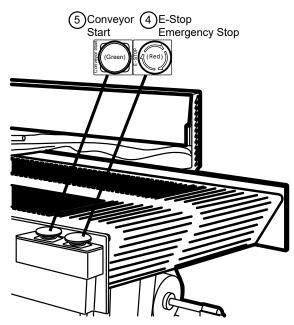
Conveyor Start — Large, green, palm button to start the conveyor for one-itemat-a-time operation. See instructions for running one product at a time later in this User Guide.
