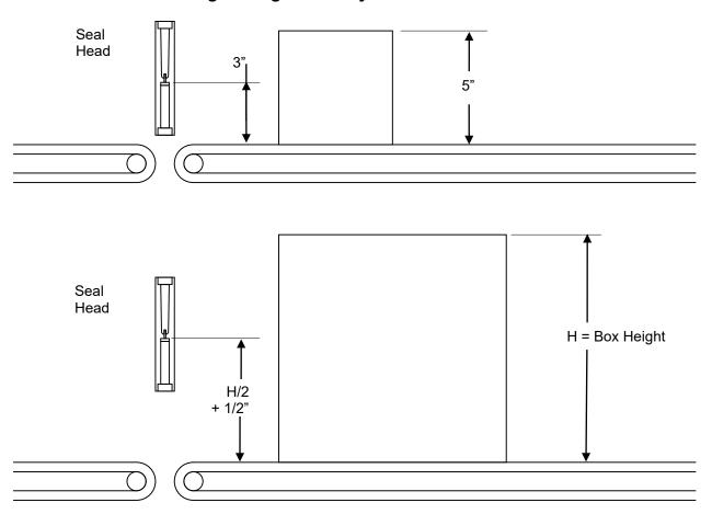
6. While adjusting the seal head height, also change the scrap chain and pinch roller height accordingly. Use the scrap chain height adjustment handle near the center of the Machine Direction seal / cutter to adjust the scrap up or down as needed.
