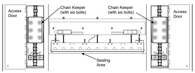
5. On the control panel side of the machine, below the access door, slowly turn the seal head adjustment knob in or out to raise or lower the seal system to the required height.
