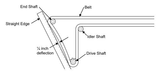
4. When the conveyor tension is correctly adjusted, re-tighten the lock nuts.
