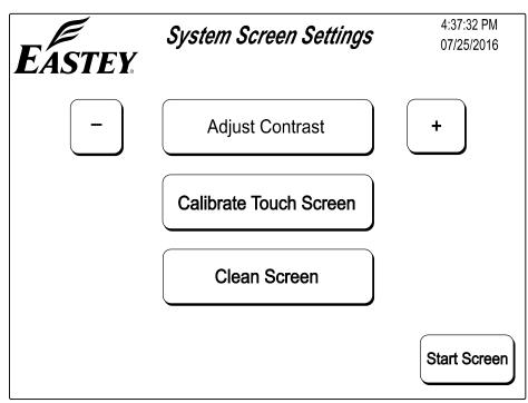
To access the System Screen Settings, touch System Settings from the System Information screen, which is displayed after the system boots up.
