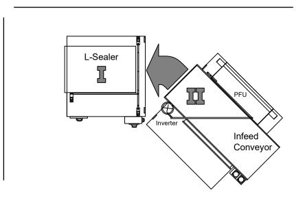
Adjust the leveling legs to support the PFU/Infeed Conveyor/Inverter module and level the Infeed Conveyor so it is level with the exit conveyor, and also level along both the machine-direction axis and transverse direction axis. Carefully align holes in attachment flanges with bolt holes in machine base. Use the bolts provided to fasten the two sections together.
