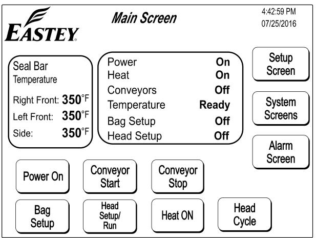
\*If your sealer is a smaller model, instead of "Right Front" and "Left Front" there may be only one heater bar, for which "Front" temperature is displayed.
