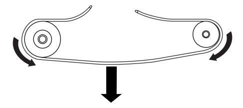
Install the new belt around the drive and idler pulleys.
