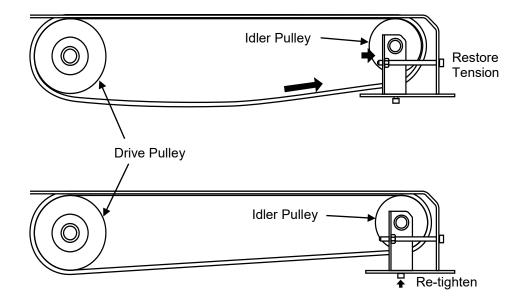
Retighten the socket head cap screws in the bottom of the conveyor to secure the idler pulley brackets in place.
