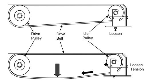
With the belt loose, remove the connecting pin that holds the belt together.
