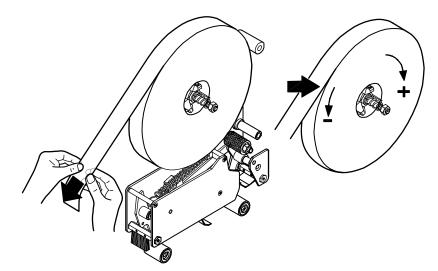
Check the tape for correct tension. Tighten or loosen the tape core holder to adjust tension.
