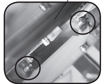
Lower fold plate seated on pins
