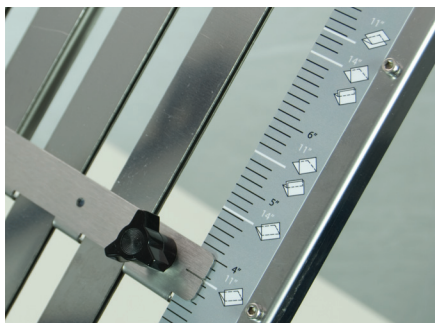
Fold stop position decal on upper fold plate.
