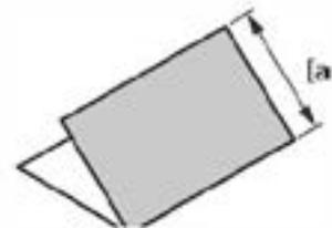
**! Incorrectly measuring the paper length or setting the folding stopper position can cause paper jamming inside the folding plate.**
