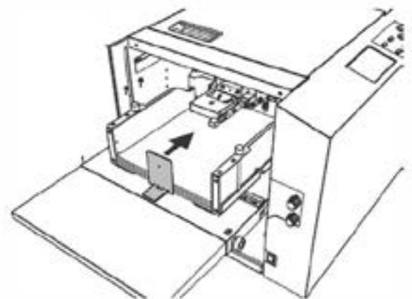
When processing long paper, use the plate unit and side guide unit.
