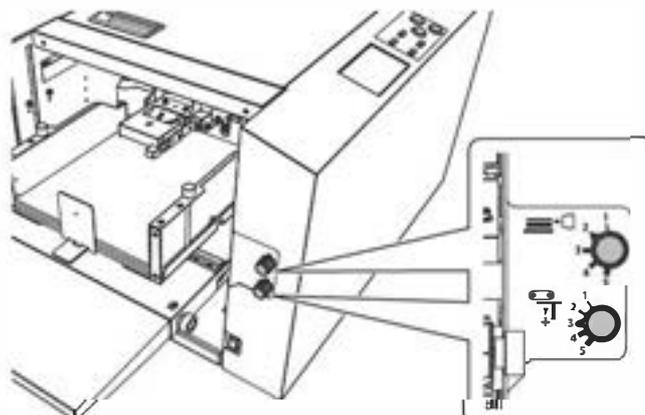
**10** Set the stack height sensor adjustment knob to the scale between the first one and second one.
