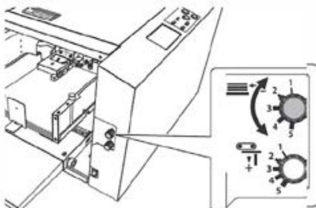
**9 Check that the separator adjustment knob is set to [2]. (The separator should be lightly in contact with the suction belt.)**
