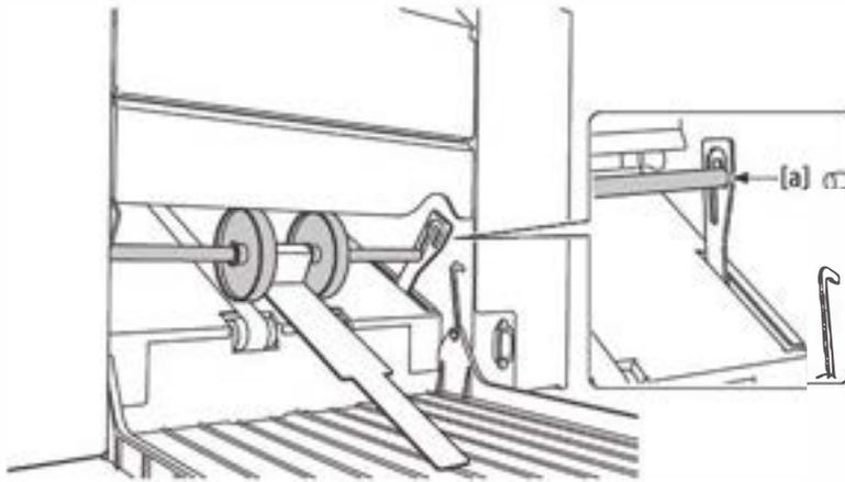
! After completing folding operations, be sure to return the stacker roller to the standard position. Leaving it in the raised state will result in poor alignment of ejected paper.
