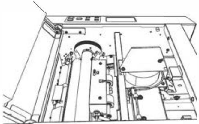
**3** Pull out the paper rotating the jam correction knob.
