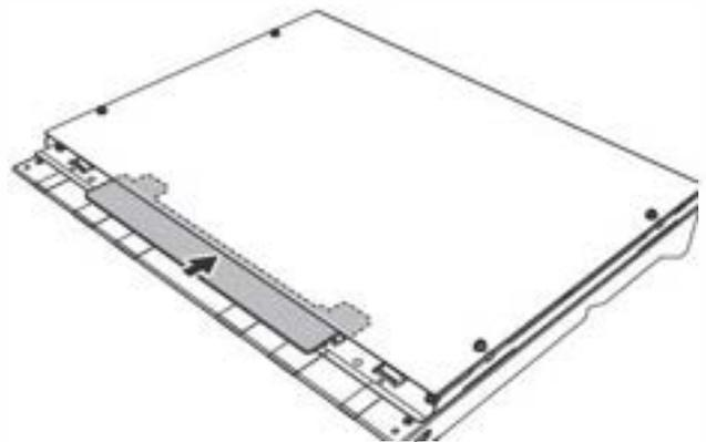
**!** Do not hold the belt section of the folding plate 2. Doing so will result in malfunction of the machine.
