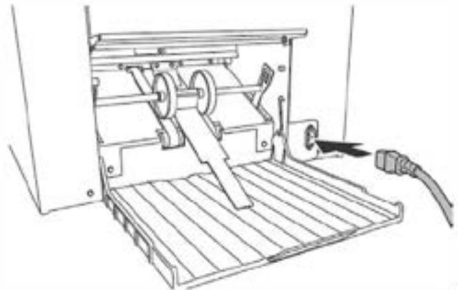
**2** Connect the power plug to the outlet with earthing connection.
