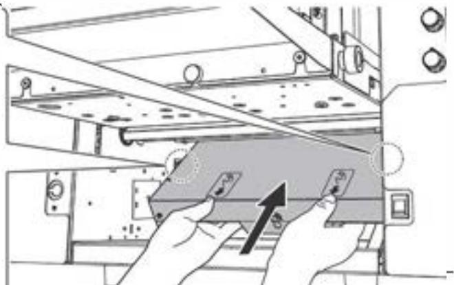
1) Insert the folding plate 2 in the direction of 1 in the right figure along with the set guide of the main body of the machine.
