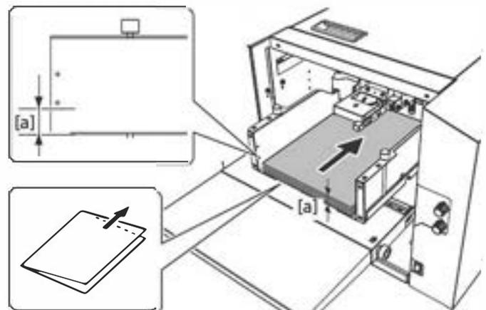
**!** A feed error may occur if the stacking height of single-folded paper is largely different on both sides even though the stacking height of single-folded paper is 25 mm/0.98 inch or less. If so, decrease the number of sheets stacked on the paper feed tray to reduce the difference on both sides of paper.
