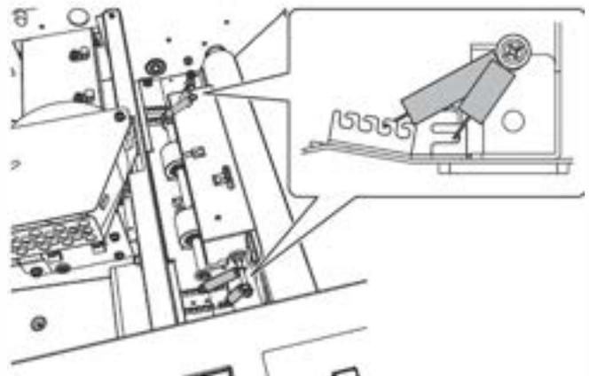
Adjust the spring pressure in the following procedures.
