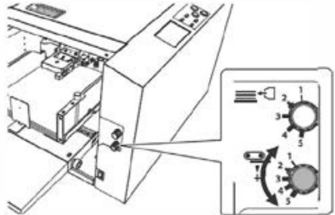
**10 Check that the stack height sensor adjustment knob is set to the standard position (the second scale from the bottom).**
