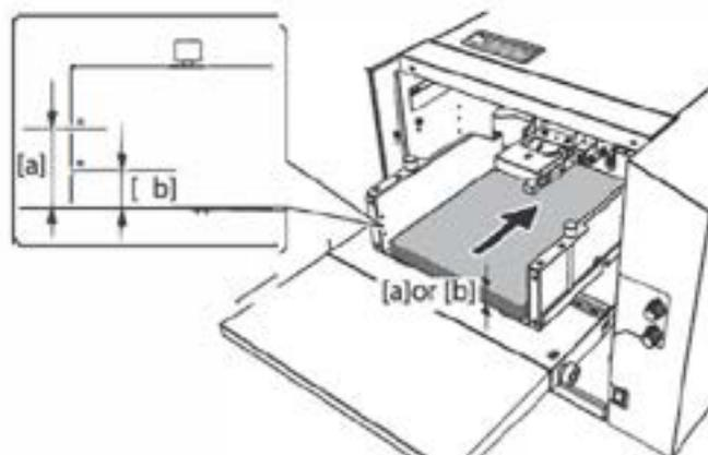
Stack paper striking the leading edge of paper lightly at the shutter. [c]
