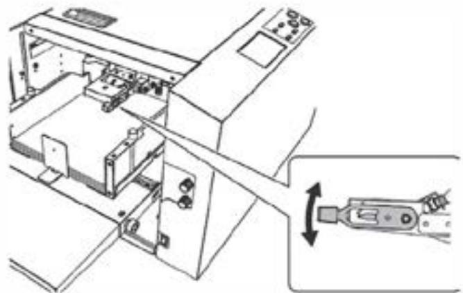
**!** A feed error may occur when stopping feeding paper with the scale of stack height sensor adjustment knob set to the first scale, and restarting feeding paper with smaller amount of paper on the paper feed tray. If so, match the stack height sensor adjustment knob with paper and set it to the following position.
