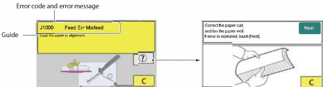
If the same error occurs frequently even when the error is solved by following the guide content, touching the **?** key displays an illustration and guide on how to solve the error.
