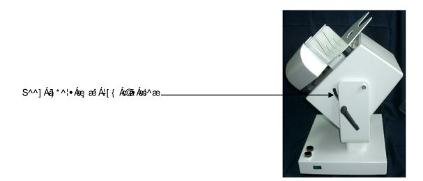
· In general, for thick paper, the tilt angle is adjusted vertically and for thin paper, it is adjusted horizontally.
