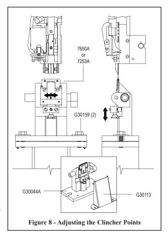
centered above the Clincher Points and the quality of the stitch will be greatly improved. Tighten the Screws to secure the Clincher Mount Assembly in this position. Complete the machine's cycle and remove the formed staple so as to not jam the Clincher Points.
