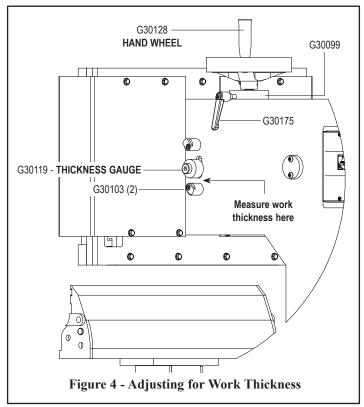
wise just enough to allow the work to be withdrawn from the Adjuster Spool, then return the Hand Wheel to the setting at which the work was clamped.
