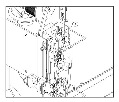
Figure 10 - Lubrication Points
