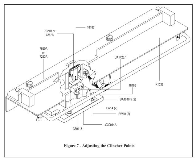
Tighten the Set Screw and replace the Clincher Guard with the Screws and Washers. Complete the cycle of the machine and test a few stitches. Repeat the previous steps if necessary.
