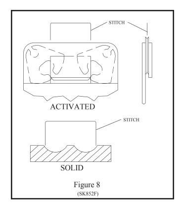
and with equal spacing from each side. When the stitch legs have penetrated the work material, the moving clinchers are raised to bend the legs towards each other and up flat against the work. The clincher points must bend both legs of the stitch against the work with the same force. Clincher points must always move freely and not bind. Dirt, wire chips, etc. will cause the points to bind.
