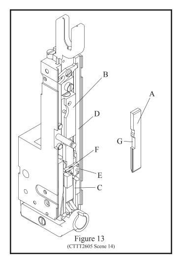
3. In conjunction with the grip release slide (Index D), it controls the movement of the bender bar latch (Index E) that opens and closes the grip (Index F).
