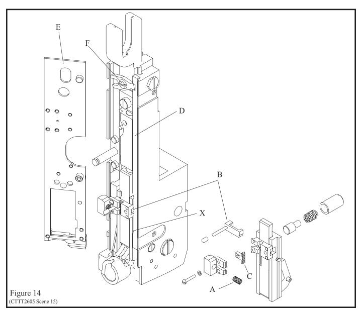
stitch. When the bender bar is stopped against the work material, the driver bar continues downward to exert pressure on the crown of the stitch, driving it through the work material.
