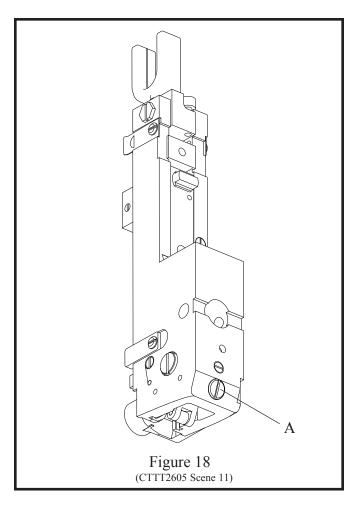
the wire points straight down as in figure 17. Improper straightening of the wire can also cause the stitch legs to buckle or turn out because they strike the clincher improperly. Excessive tension on the wire straightener prevents the grip (Index D) from feeding the wire smoothly. This causes variation in leg length.
