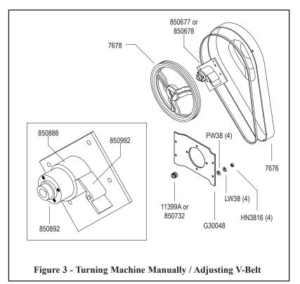
Mounting Plate to move the Plate down slightly. Pressing on the Pulley (850732) may knock it out of position. Tighten the four (4) Hex Nuts again when the V-Belt is taut. The V-Belt should first be tightened after two to three weeks of use and then periodically after that.
