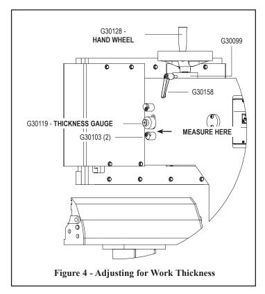
Anytime the thickness of work changes, a sample should be tested in the M27 so no serious damage is caused to the machine. If the machine is operated on work thicker than it is set to handle, damage will result and the stitcher machine will not operate properly.
