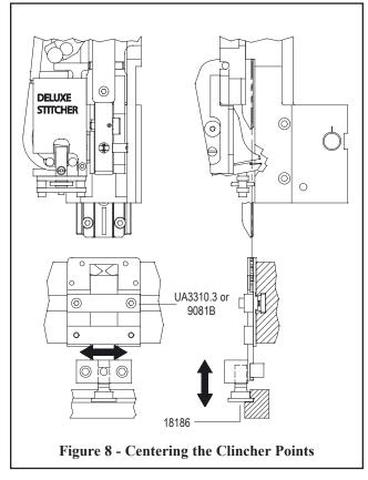
from back to front. Tighten the Screws to secure the Clincher Rail in this position. Re-check the side-to-side adjustment after completing the front-to-back
