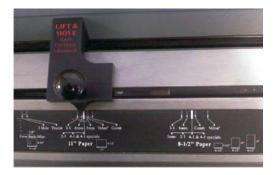
paper stop can now be made by turning the knob on the left side of the HD7700/H to move the paper stop left or right until the punch pattern is centered on the paper.
