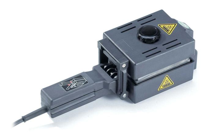
The PF-100S is a hot-pressing device for Flexproof joining of Habasit belts and tapes up to a width of 100 mm / 4 in. and a thickness of 2.5 mm / 0.10 in.. The lower press plate is heated and is equipped with a integrated overheating fuse and temperature regulator. Its knuckle joint mechanism allows easy adjustment for different belt thicknesses. Together with the integrated pressure equalization pad, it ensures reliable hot pressing of fusion joints.
