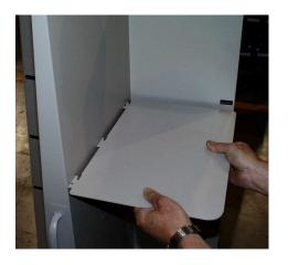
Lift the shelf slightly so the bent tab will clear the hole edges and slide the shelf into the truck body.
