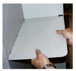
Drop the shelf down so the bent tab is seated in the frame hole.
