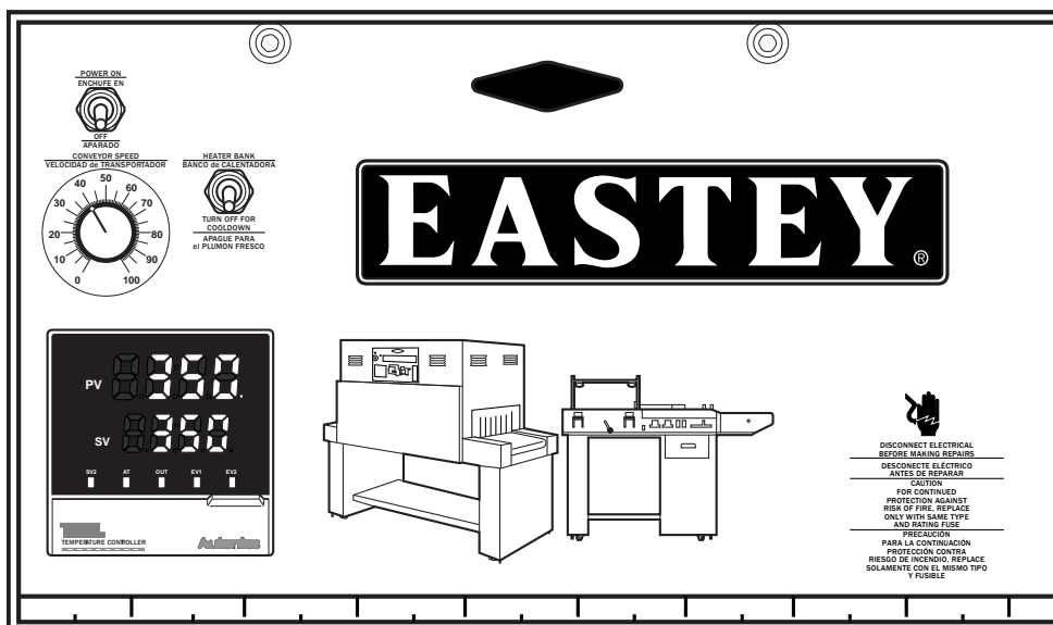
Control Panel for units manufactured previously and up to 2015.
