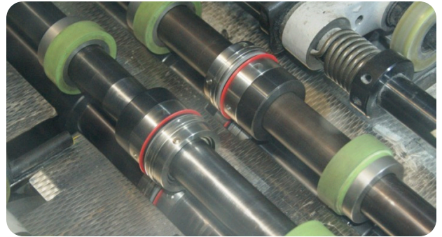
Quad HD TS30 heads installed on a binder cover feeder.
