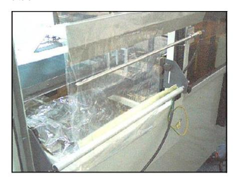
6. Pull the film out slightly more than one meter (39 inches) across the top of the upper inverter.
