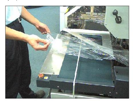
8. Unfold and open the film, holding the top film across the top of the upper inverter triangle with your left hand, so the film enters, top film over the top to flip underneath. With your right hand, bring the bottom film underneath the infeed conveyor at the infeed end and underneath the bottom inverter so the bottom film enters under the bottom to flip over to the top side of the bottom inverter. See the following illustration on the next page.
