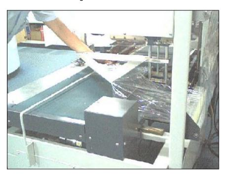
11. Pull the film to the left to the L-sealing area and lift the lever to temporarily release the pinch wheels.
