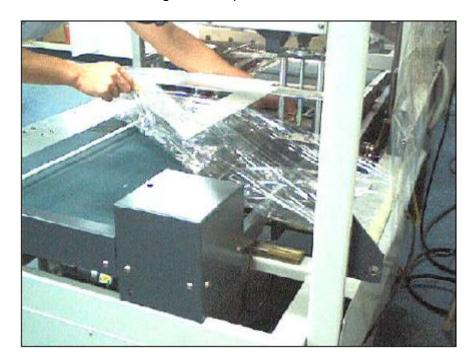
10. Match both the top sheet and bottom sheet of the film and guide the leading end of the film toward the sealing area.
