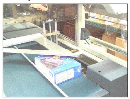
2. Adjust the height of the Film Guide Roller (shown in the photo below) to the center of the distance between the upper and lower triangles of the film inverter. Refer to the illustration on the following page.
