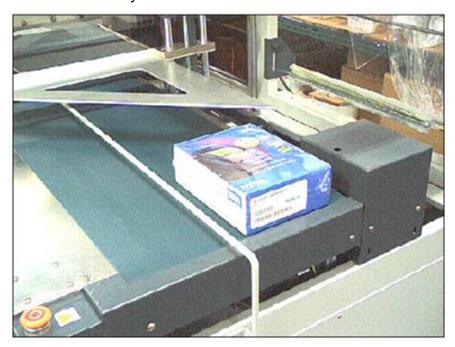
2. Place the product against the rear edge of the Infeed conveyor as shown below, and measure the height
