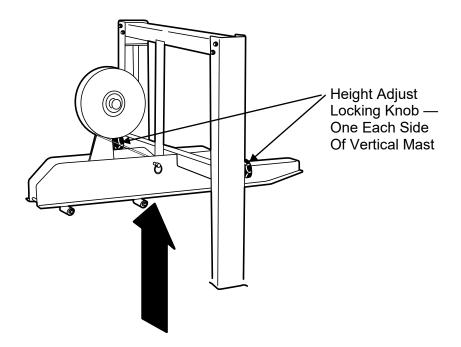
After raising the top taping head up, remove the lower taping cartridge from the bottom section by holding both lift points and lifting leading with the rear lift point first, raising the tape cartridge upward, out of the lower tape head seat.
